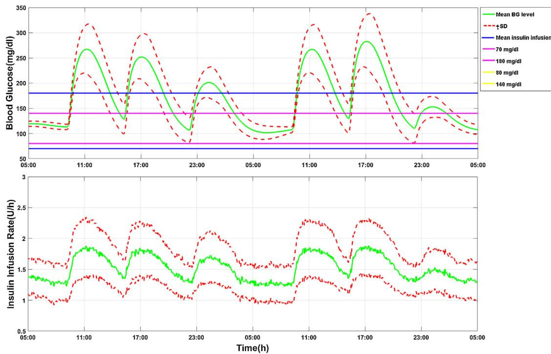
**Fig. 5.** Response of the mean blood glucose regulation (green solid line) and standard deviation (red dotted line) with the corresponding mean insulin infusion rate (blue solid line) and standard deviation (red dotted line) for scenario 2. Yellow solid line represents 80 mg/dl and 140 mg/dl. Magenta solid line represents 70 mg/dl and 180 mg/dl. (For interpretation of the references to color in this figure legend, the reader is referred to the web version of the article.)
