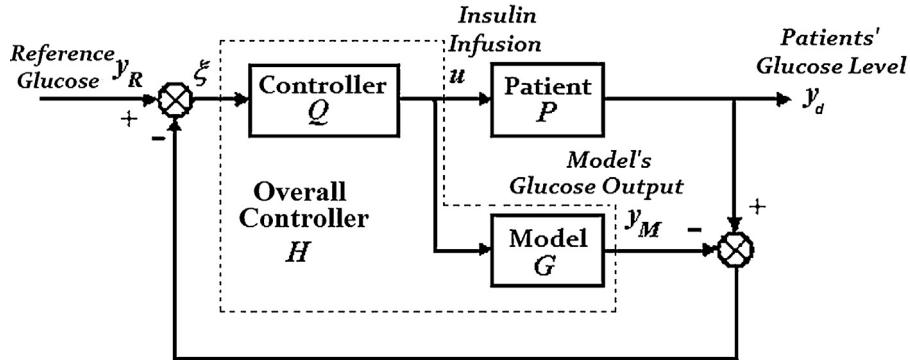
**Fig. 1.** Structure of an IMC based artificial pancreas system.**Table 2**
