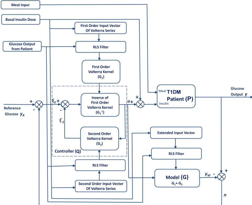
**Fig. 2.** Block diagram of online-tuned internal model control scheme.
