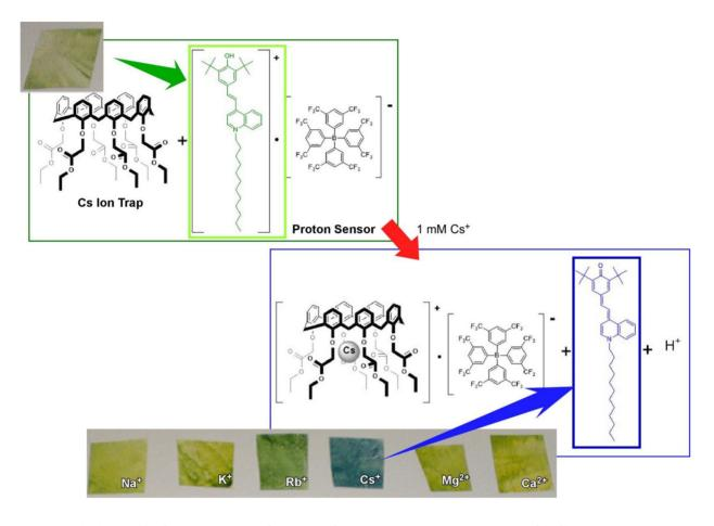
Figure 9. Supramolecular assembly of optode sensor system for detection of Cs ions in solution through color changes of the film.
