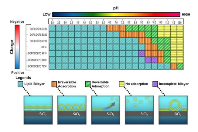
Figure 5. QCM—D measurement profiling of vesicle adsorption onto a silicon dioxide surface. Experiments were conducted as a function of solution pH and membrane surface charge (by varying the lipid composition). DOPC, DOPS, and DOEPC are neutral, anionic, and cationic phospholipids, respectively. The color scheme in each box corresponds to the measured morphological properties of the resulting lipid adlayer. Reprinted with permission from Ref. [56]. Copyright 2018 American Chemical Society.
