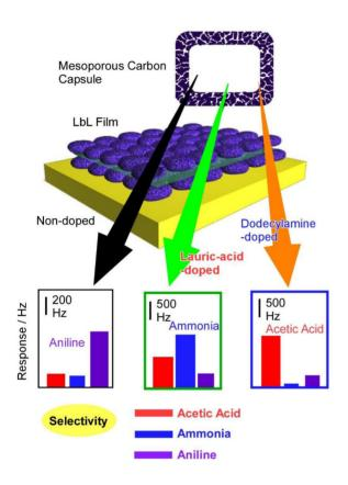
**Figure 3.** Layer-by-layer films of mesoporous carbon capsules with polyelectrolyte on a QCM sensor electrode whereby selectivity can be altered through impregnation of the second recognition component within the capsule structure.
