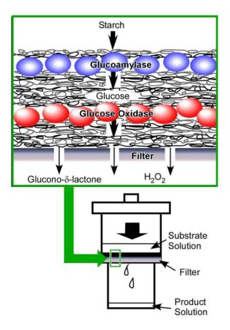
**Figure 4.** Layer-by-layer enzyme reactor from starch to gluconolactone via glucose with upper layer of glucoamylase (for conversion of starch to glucose) and bottom layer of glucose oxidase (from glucose to gluconolactone) on ultrafilter reactor.
