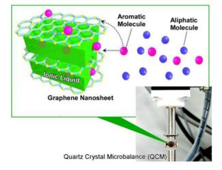
Figure 2. Layer-by-layer assemblies of graphene and ionic liquid layers on a QCM sensor for toxic (aromatic) gas sensing.
