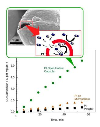
**Figure 10.** Micrometer-sized hollow Pt cells (metallic cells) for agglomeration-tolerant catalytic performance of CO remediation (CO+ $1/2O_2 \rightarrow$  CO<sub>2</sub>): green, metallic cell (Pt open hollow capsule); brown, Pt on microsphere; black, Pt powder.
